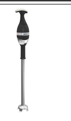
602237 (DBP6565U) Portable mixer, hand held immerson blender, variable speed, handle grip, with 26" tube, 1 HP, 650 W, NEMA 5-15P plug
