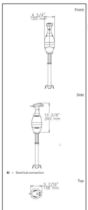
Electric Supply voltage: 110-120 V/1 ph/50/60 Hz **Total Watts:** 0.65 kW Plug type: USA NEMA 5-15P Key Information: External dimensions, Width: 5 7/16" (138 mm) External dimensions, 4 3/4" (120 mm) Depth: External dimensions, 38 " (965 mm) Height: **Shipping width:** 11 7/16" (290 mm) Shipping depth: 27 3/16" (690 mm) Shipping height: 7 1/16" (180 mm) **Shipping weight:** 13 lbs (5.7 kg)
